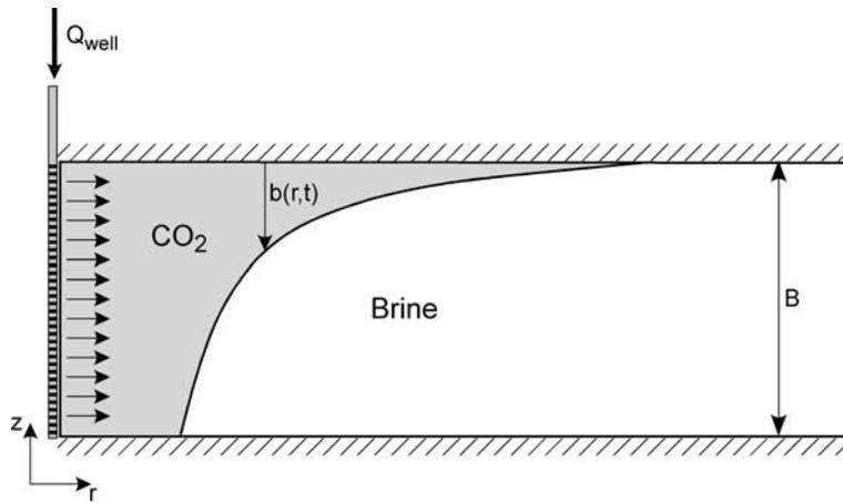
**Figure 5:** Typical profile of CO<sub>2</sub> plume defined by thickness  $b(r,t)$ .
