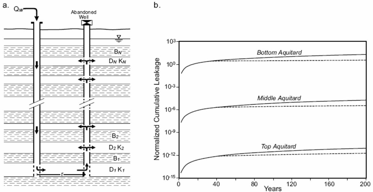
**Figure 4:** (a) Schematic showing injection well and leaky well in a multi-layer system, and (b) Cumulative leakage rates, normalized by amount injected, for leakage through the lowest aquitard, the middle aquitard, and the upper-most aquitard, in a domain with 11 aquifers and 10 aquitards, with solid line representing continuous injection and dashed line representing injection for the first 30 years (taken from [17]).
