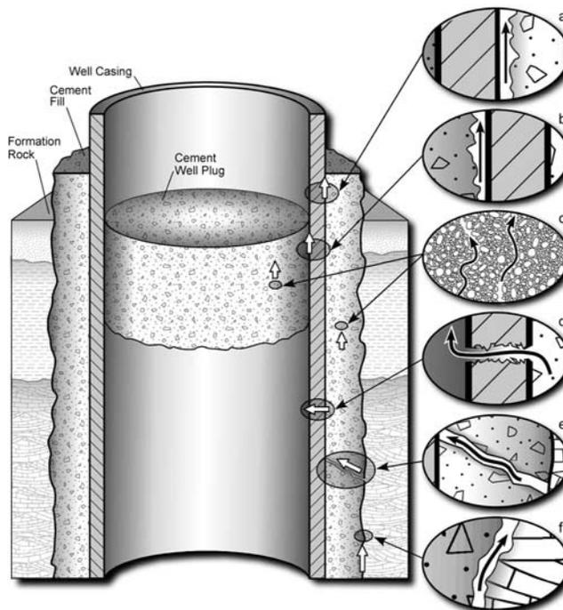
**Figure 2:** Potential leakage pathways along an existing well: between cement and casing (paths a and b), through the cement (c), through the casing (d), through fractures (e), and between cement and formation (f).
