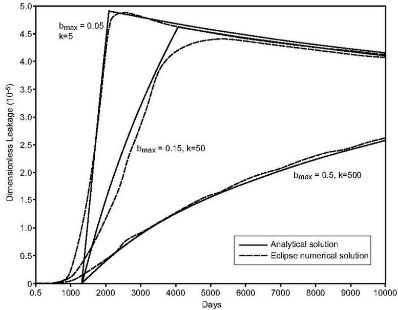
**Figure 6:** Leakage rate of CO<sub>2</sub> through an abandoned well, for three different permeability values assigned to the leaky well. Dimensionless leakage is leakage rate divided by injection rate, normalized by the ratio of formation permeability to leaky-well permeability. Best-fit values of the parameter  $b_{max}$  are shown for each curve. Leaky-well permeability values are shown for each curve in units of Darcy.
